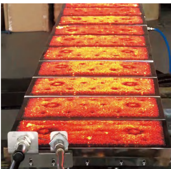
Infrared Heating Equipment
